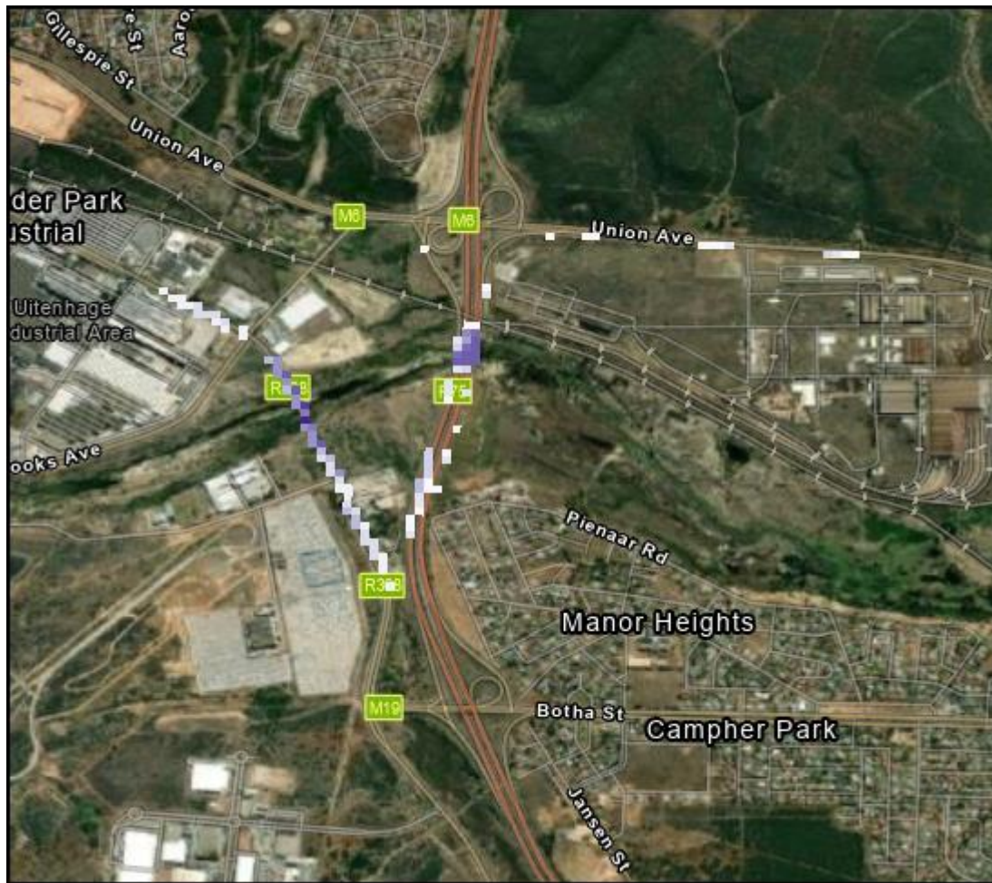
Figure: Roads affected by 8m inundation
